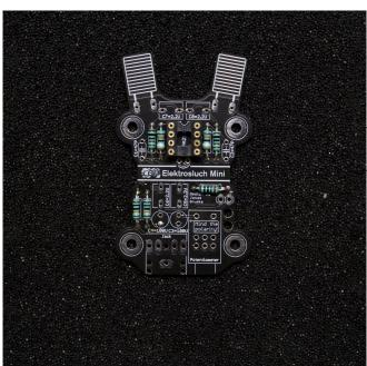
3. **Continue with the socket for the integrated circuit.** Note its orientation, marked by the little U-shaped cutout. This cutout should be pointed to the top. Using a socket is good practice when dealing with chips - it allows you to swap the chip for another one for altering the performance of the circuit, and protects the chip from damage during the soldering stage.
