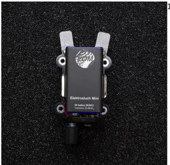
18. Insert the battery into the holder.
