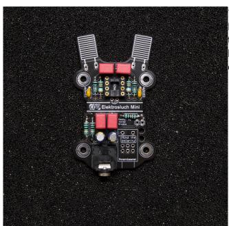
7. **Solder in the two electrolytic capacitors.** Beware of their polarity, minus (-) is marked on the body and plus (+) is marked on the circuit board! Double check you are soldering them in correctly, it isn't easy to desolder them.
