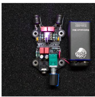
12. Solder in the LED. Use the provided heatshrink tubing to cover the LED legs. The longer leg goes into to the right side hole. Once placed, bend the LED as you see fit.
