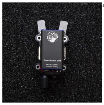
18. Insert the battery into the holder.
