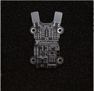
mostly placing components (from the top side!) in the correct places and soldering them from the underside of the circuit board. After each soldering stage, you can cut off the leads of the components with side cutters, so they're not in the way.
