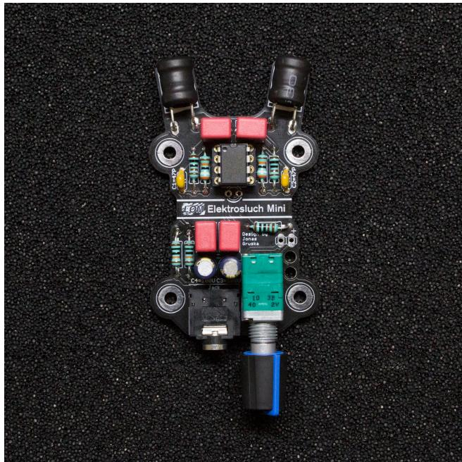
**11. Pop-in the integrated circuit chip into the socket.** Make sure you're placing it with the U shaped cutout towards to the antennae, as pictured. It might be necessary to change the angle of its legs so they fit snuggly. You can realign them easily by pressing them against a table.
