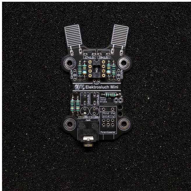
5. Then the yellow **ceramic capacitors** marked as 470 (47 pF). These will help to protect the circuit from very high frequencies beyond the audible range and oscillations. These are not polarity sensitive.
