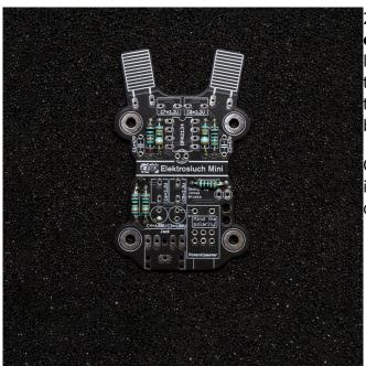
2. It is best to **start soldering the shortest components first** and then move on to the larger ones. After you place the component legs through the holes, it may be handy to bend them in such a way that it wont fall out when the board is flipped over for soldering.
