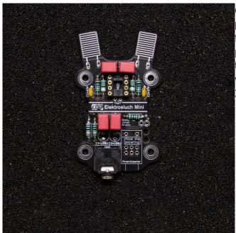
6. Now you can solder in the 4 pink polypropylene capacitors. These will limit low frequency pick-up. These capacitors are also not polarized. Also if you decide that you would like to have bit more bass, you can replace these with higher values (for example 10  $\mu$ F instead of 2.2  $\mu$ F).
