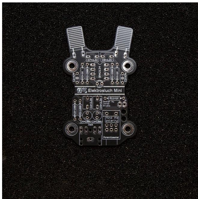
mostly placing components (from the top side!) in the correct places and soldering them from the underside of the circuit board. After each soldering stage, you can cut off the leads of the components with side cutters, so they're not in the way.
