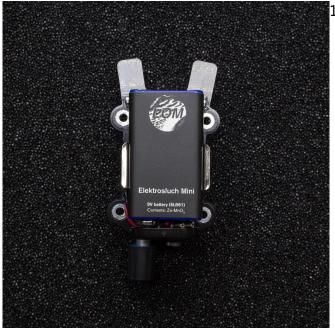
18. Insert the battery into the holder.
