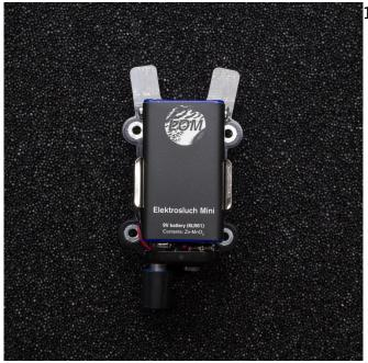
18. Insert the battery into the holder.
