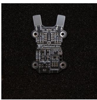
1. Examine the printed circuit board. You can see that it is covered with markings, indicating the correct placement of the components. During this tutorial, you will be mostly placing components (from the top side!) in the correct places and soldering them from the underside of the circuit board. After each soldering stage, you can cut off the leads of the components with side cutters, so they're not in the way.
