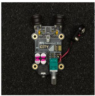
Pull the wires through the hole next to the potentiometer as pictured and solder them in.
