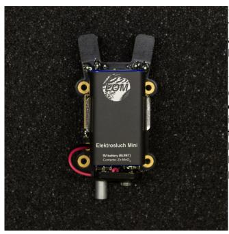
13. Cover the battery with attached LOM sticker. This protects from parts on the board accidentaly shorting on the battery metallic body.
