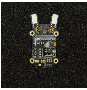
3. Continue with the yellow **ceramic capacitors** marked as 100 (10 pF). These will help to protect the circuit from very high frequencies beyond the audible range and oscillations. These are not polarity sensitive.
