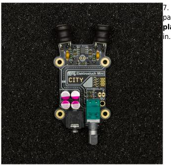
7. Remove the protective film from the sticky pads on the "antennae" of the circuit board and **place the inductors** as pictured. Solder them
