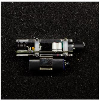
17. Eleketrosluch Mini City kits shipped at the end of September 2017 and onwards have **extra acrylic cover** for the bottom of the circuit board. Attach it as pictured.
