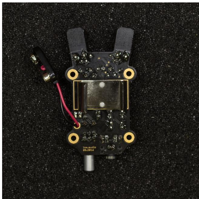
**18. Insert the battery into the holder.**
