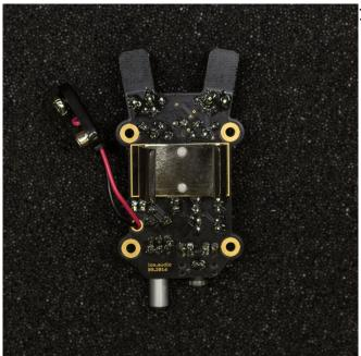
18. Insert the battery into the holder.
