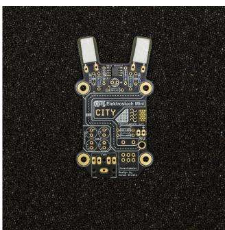
1. Examine the printed circuit board. You can see that it is covered with markings, indicating the correct placement of the components. During this tutorial, you will be mostly placing components (from the top side!) in the correct places and soldering them from the underside of the circuit board. After each soldering stage, you can cut off the leads of the components with side cutters, so they're not in the way.
