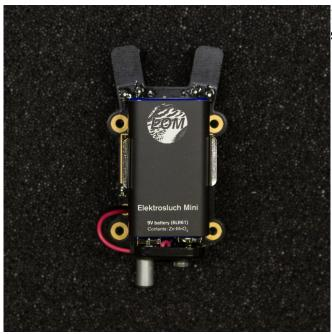
19. Attach the front cover using the 8 screws and 4 stand-offs.
