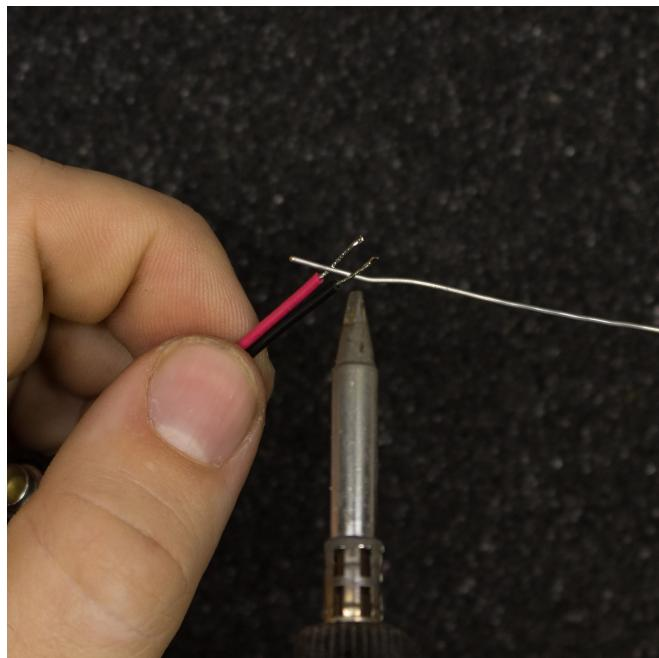
11. Pull the wires through the hole next to the potentiometer as pictured and solder them in. Thi
