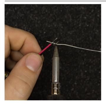
Pull the wir es thr ou gh the hol e ne xt to the pot ent io me ter as pic tur ed an d sol der the m in. Thi
