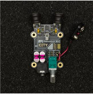
11. Pull the wires through the hole next to the potentiometer as pictured and solder them in. This will act as a strain relief for the connection. The red lead goes to the plus and black to the minus.
