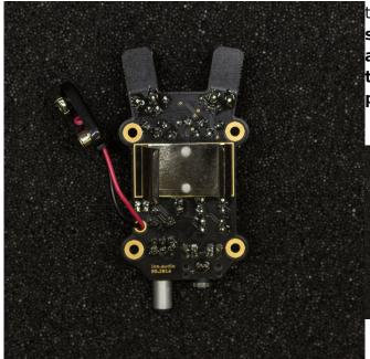
the bottom. Make sure that leads are cut as short as possible, so they won't make accidental contacts with the holder. Use the tape to attach the holder as pictured.</WRAP>
