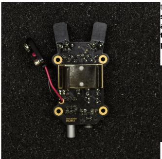
the bottom. Make sure that leads are cut as short as possible, so they won't make accidental contacts with the holder. Use the tape to attach the holder as pictured.</WRAP>
