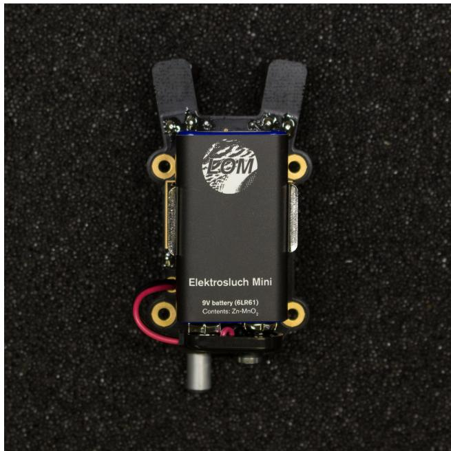
13. (Optional) Cover the battery with attached LOM sticker. 14. **Check one more time if all the polarities (capacitors, battery connector, battery) are correct.** Reversing the polarity might irreversibly damage the circuit. Attach the battery and turn on the device with the potentiometer (it has a built-in switch!).
