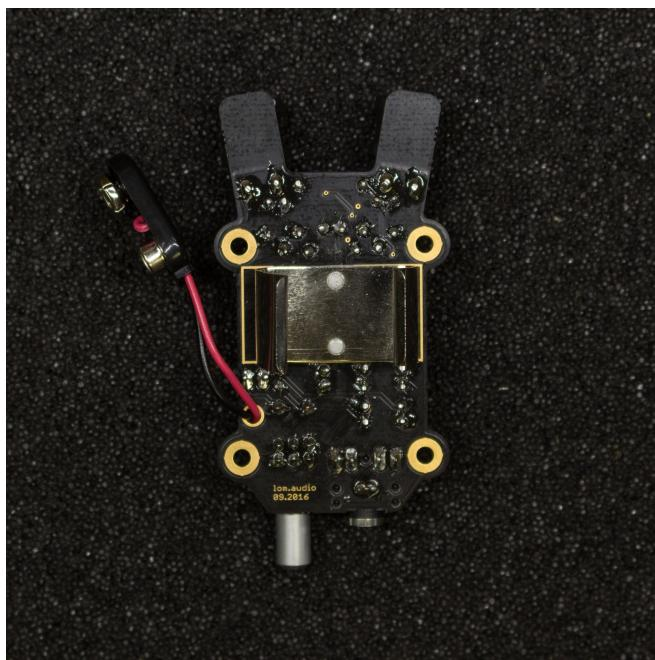
**holder to the bottom.** Make sure that leads are cut as short as possible, so they won't make accidental contacts with the holder. Use the tape to attach the holder as pictured.
