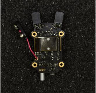
**holder to the bottom.** Make sure that leads are cut as short as possible, so they won't make accidental contacts with the holder. Use the tape to attach the holder as pictured.
