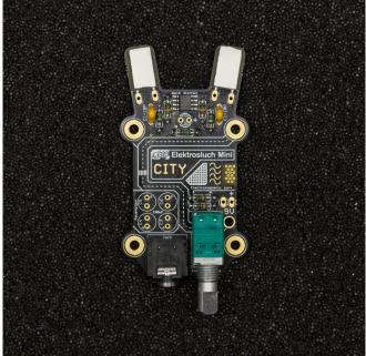
5. Push the **potentiometer** onto the board until it snaps into place and solder it in.
