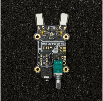
5. Push the **potentiometer** onto the board untilit it snaps into place and solder it in.
