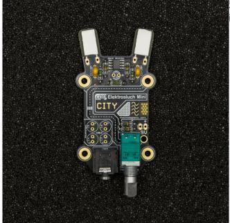
5. Push the **potentiometer** onto the board untilit it snaps into place and solder it in.
