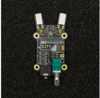
5. Push the **potentiometer** onto the board until it snaps into place and solder it in.
