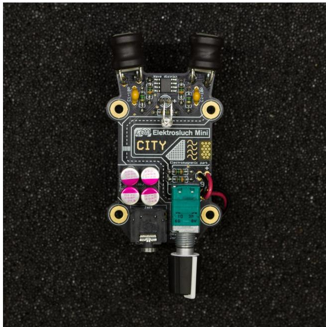
15. Put the **knob** on the potentiometer. It requires a bit of pressure, make sure you're holding the pot and pressing it against it, not against the whole device.
