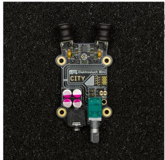
7. Remove the protective film from the sticky pads on the "antennae" of the circuit board and **place the inductors** as pictured. Solder them in.
