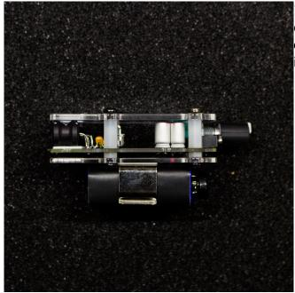
17. Eleketrosluch Mini City kits shipped at the end of 2017 and onwards have **extra acrylic cover** for the bottom of the circuit board. Attach it as pictured.
