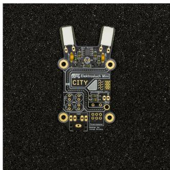
3. Continue with the yellow **ceramic capacitors** marked as 100 (10 pF). These will help to protect the circuit from very high frequencies beyond the audible range and oscillations. These are not polarity sensitive.
