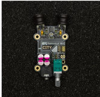
7. Remove the protective film from the sticky pads on the "antennae" of the circuit board and **place the inductors** as pictured. Solder them in.
