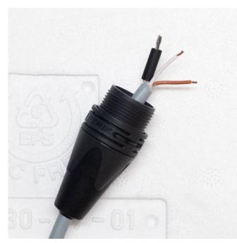
2. Unpack the XLR connector and the small piece heat-shrink tubing from the tube. Identify the cable end with three leads. **Slide on the XLR boot** (if you forget, you may need to desolder the connector later) on the cable and the small piece of heat-shrink tubing on the exposed twisted conductor without the insulation — this is the shielding of the cable.
