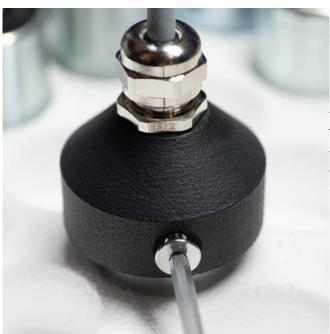
8. Carefully pull the cable with the element soldered on through the gland as far as possible (without damaging the solder joints). Use the provided bolt (in the tube) and a 2.5 mm Allen (hex) key to fix the element in position through the side hole on the top part of the Geofón body. The thread is only 3D printed, so be careful not to over-tighten. The main purpose of this bolt is to prevent the Geofón element from rotating when the body is disassembled.
