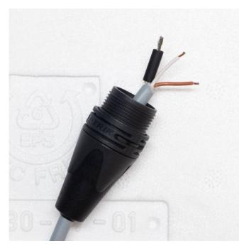
2. Unpack the XLR connector and the small piece heat-shrink tubing from the tube. Identify the cable end with three conductors. Slide the XLR boot onto the cable (if you forget, you may need to desolder the connector later) and the small piece of heat-shrink tubing onto the exposed twisted conductor without insulation—this is the cable's shielding.
