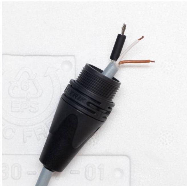
2. Unpack the XLR connector and the small piece heat-shrink tubing from the tube. Identify the cable end with three conductors. Slide the XLR boot onto the cable (if you forget, you may need to desolder the connector later) and the small piece of heat-shrink tubing onto the exposed twisted conductor without insulation—this is the cable's shielding.
