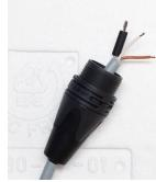
2. Unpack the XLR connector and the small piece heat-shrink tubing from the tube. Identify the cable end with three conductors. Slide the XLR boot onto the cable (if you forget, you may need to desolder the connector later) and the small piece of heat-shrink tubing onto the exposed twisted conductor without insulation—this is the cable's shielding.
