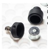
5. Unscrew the Geofón body parts apart and remove the Geofón element from inside.
