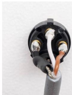
3. solder the provided XLR connector to the cable. You'll notice it has small number markings. Solder the exposed conductor with heat-shrink tubing to pin number 1, the brown conductor to pin 2, and the white conductor to pin 3. The heat-shrink tubing will shrink as you solder
