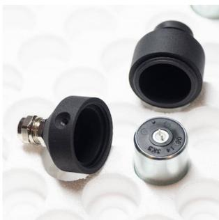
5. Unscrew the Geofón body parts apart and remove the Geofón element from inside.
