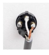
3. older the provided XLR connector to the cable. You'll notice it has small number markings. Solder the exposed conductor with heat-shrink tubing to pin number 1, the brown conductor to pin 2, and the white conductor to pin 3. The heat-shrink tubing will shrink as you solder
