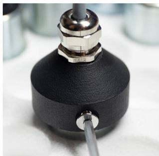
8. Carefully pull the cable with the element soldered on through the gland as far as possible. Make sure you won't damage the solder joints. Use the provided bolt (in the tube) and a 2.5 mm Allen (hex) key to fix the element in position through the side hole on the top part of the Geofón body. The thread is in the plastic material, so be careful not to over-tighten as you may strip it.
