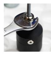
9. Screw the bottom part of the Geofón body onto the top part, and tighten the cable gland on top of the top part of the Geofón as tightly as possible by hand. If necessary, use a 14 mm wrench, but do not overstrain the gland. If you encounter difficulties while screwing the bottom part of the body, check if the side bolt is
