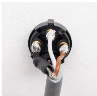
3. Solder the provided XLR connector to the cable. You'll notice it has small number markings. Solder the exposed conductor with heat-shrink tubing to pin number 1, the brown conductor to pin 2, and the white conductor to pin 3. The heat-shrink tubing will shrink as you solder
