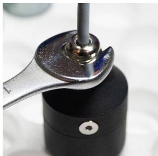
9. Screw the bottom part of the Geofón body onto the top part, and tighten the cable gland on top of the top part of the Geofón as tightly as possible by hand. If necessary, use a 14 mm wrench, but do not overstrain the gland. If you encounter difficulties while screwing the bottom part of the body, check if the side bolt is
