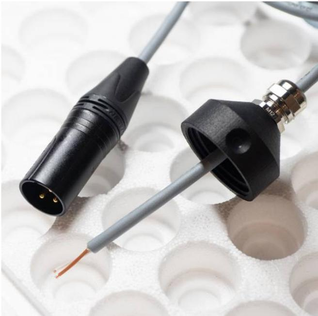
7. Tin the exposed conductors on the cable with a bit of solder. Solder the conductors to the pins on the element. Brown conductor should be connected to the pin with a dot next to it. Solder as fast as possible, one joint shouldn't take longer then 2-4 seconds (depending on your soldering iron).
