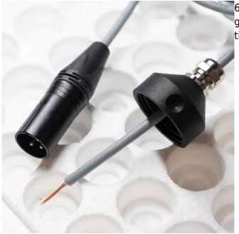
Pull the unused cable end through the cable gland on the top part of the Geofón body. Do not tighten the gland yet!
