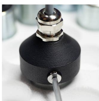
8. Carefully pull the cable with the element soldered on through the gland as far as possible. Make sure you won't damage the solder joints. Use the provided bolt (in the tube) and a 2.5 mm Allen (hex) key to fix the element in position through the side hole on the top part of the Geofón body. The thread is in the plastic material, so be careful not to over-tighten as you may strip it.
