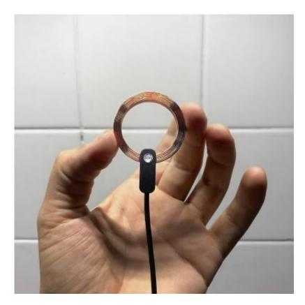
Elektroucho Pro is a mono, passive electromagnetic sensor. You can use with as a regular dynamic microphone with a standard XLR preamplifier. It is significantly more sensitive than other common electromagnetic pickups (such as telephone pickup coils). It is more sensitive than our Elektrouši.
