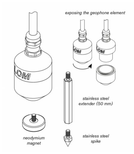
**Geofón** is a sensitive geophone adjusted for field recording purposes. Originally designed for seismic measurements, it can be used with regular field recording equipment to capture very faint vibrations in various materials and even soil.
