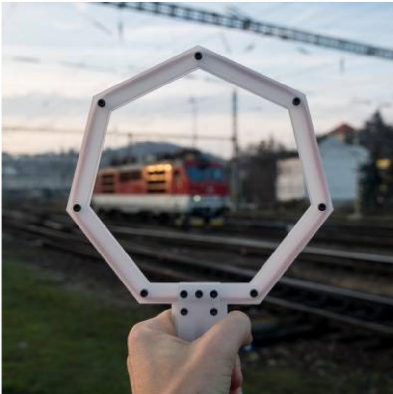
Priezor is an open-source passive magnetic antenna for electromagnetic listening. It is very sensitive and capable of capturing faint atmospheric events in VLF radio bands. Compared to regular Elektroschluch, it is less directional and focused, and therefore more useful in recording ambient electromagnetic fields, where the overall “sound of the place” is desired.
