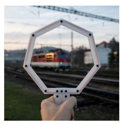
Priezor is an open-source passive magnetic antenna for electromagnetic listening. It is very sensitive and capable of capturing faint atmospheric events in VLF radio bands. Compared to regular Elektrosluch, it is less directional and focused, and therefore more useful in recording ambient electromagnetic fields, where the overall "sound of the place" is desired.
